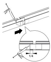
**4.** Insert the second gutter ¼ of the way into the other side of the gutter extenstion and put sealant on the edges.
