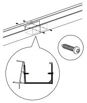
**6.** The gutter extension can now be secured with the short stainless steel screws in the chamber of the gutter and on the front side under the decorative profile. Put sealant on the assembly so it is smooth and waterproof!
