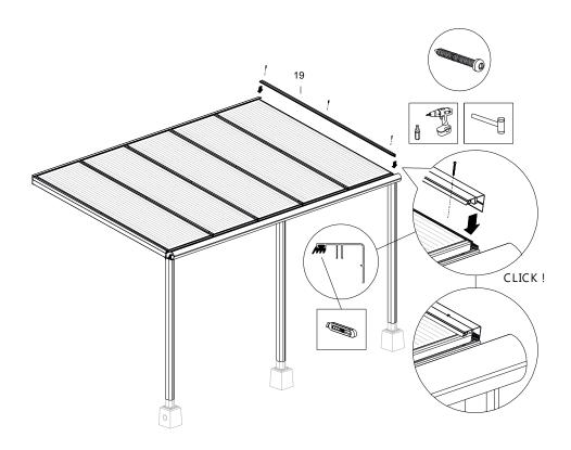
**11.** Now screw a sheet stopper at the gutter end of each middle beam to ensure secure attachment. **Note:** securing the end cover strips comes later.
