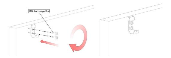
**3.** Install the wall profile on the wall mounting brackets.
