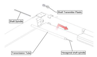
**5.** Insert a shaft transmitter plastic on to the transmission tube on the inside of the system.
