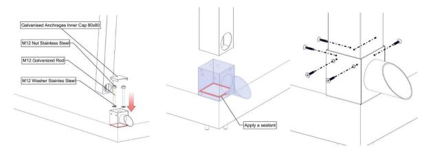
**9.** Slide the rubber flap in and place gutter cover and fasten the screws.
